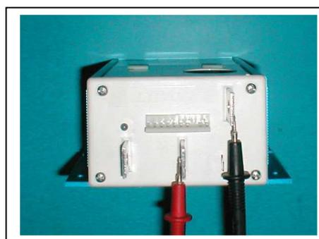
Meter should be reading 0.5V ± 0.2V
