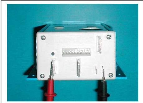
Meter should be reading  $0.5V \pm 0.2V$
