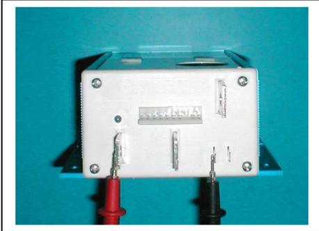
Meter should be reading  $0.5V \pm 0.2V$
