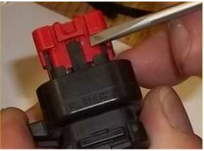
Pull the red cap upward  $\frac{1}{4}$ " – it will stop, this is the UNLOCKED POSITION
