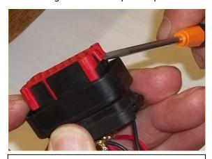
Very carefully pry the red clip upward, it will unclick. This tab can break to be careful!
