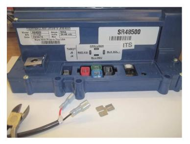
The FN Function box requires KSI voltage input, so we use the supplied TAB-TAP to connect both Key Switch Input and the FN Box power.
