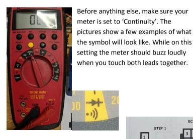
To test the board level connections of the controller, we have to measure continuity between the red squares of each step. The multimeter should give a loud buzz/beep to confirm we have a good internal connection.
