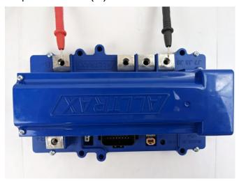
Meter should be reading  $0.5V \pm 0.2V$
