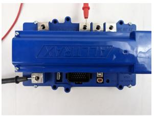
Meter should be reading  $0.5V \pm 0.2V$
