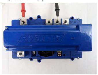
Meter should be reading  $0.5V \pm 0.2V$
