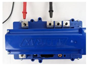
Meter should be reading  $0.5V \pm 0.2V$
