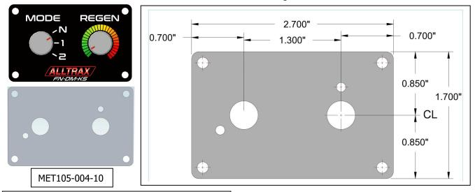
Check behind the panel to ensure you won't drill into wiring or other critical things. Measure twice – drill once!
