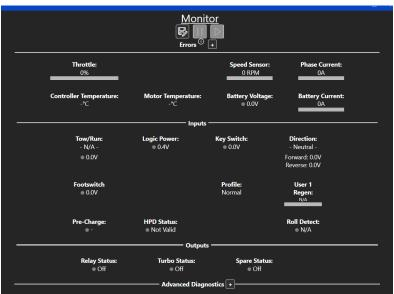
The three buttons at the top of the screen allow you to save your monitor log to a file, Pause recording and Start recording.
