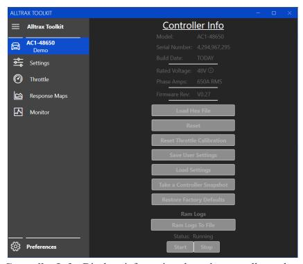
**Controller Info:** Displays information about the controller such as rated voltage, RMS current rating, serial number, build date and which firmware revision it is using.
