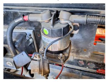
4. Remove wires and unplug wire harness, then remove the bolts holding the motor controller heatsink assembly. Remove from car:
