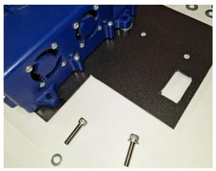
7. Install the new Solenoid with the terminals facing up using the two 1/4-20x1" HEX HEAD bolts with 1/4" FLAT Washers.
