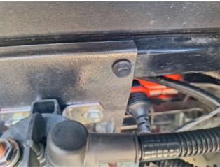
13. Install and connect the 3-phase motor wires as shown with U, V, W going to the correct terminals. U=BLK-TOP / V=RED-CENTER / W=WHT-BOTTOM. Torque bolts to specs on AC1 Manual **SPECIFICATIONS SECTION**. ZIP Tie the cable assembly using the OEM ring support shown above the motor.
