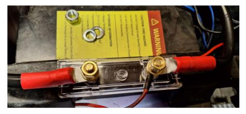
2. Connect cable 5/16" ring to the fuse, the 3/8" ring to the 400amp solenoid.
