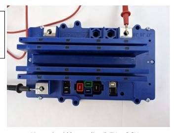
Meter should be reading  $0.5V \pm 0.2V$
