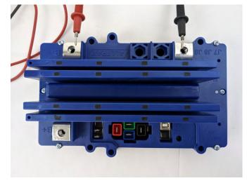
Meter should be reading  $0.5V \pm 0.2V$
